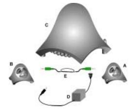
Connect the speaker system as shown in the **Connecting the speaker system to sound card** illustrations. Once the speaker system is properly connected, turn on the power switch located on the rear of the subwoofer.
